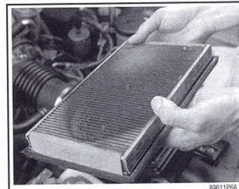
Fig. 46 An example of a severely clogged filter element. A filter this dirty can hamper engine performance
