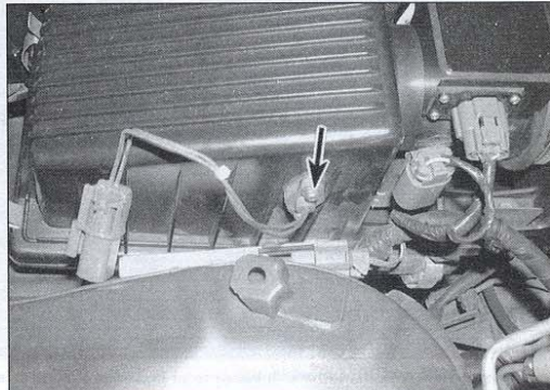
7.3a Disconnect the electrical connector from the intake air temperature sensor (arrow) and measure the resistance across the two terminals of the sensor connector
