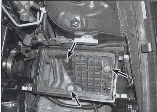
9.5 Remove the bolts (arrows) and the lower air filter housing
