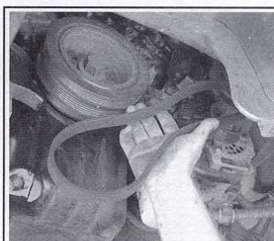
Fig. 77 The replacement of some belts may require the removal of other belts
