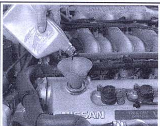
Fig. 152 Add oil in small increments; overfilling the engine with oil can damage internal components
