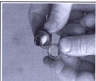
Fig. 156 The copper washer should be replaced to ensure a leak-free seal
