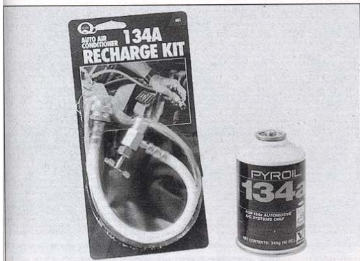
12.18 A basic charging kit for 134a systems is available at most auto parts stores - it must say 134a (not R-12) and so should the can of refrigerant
