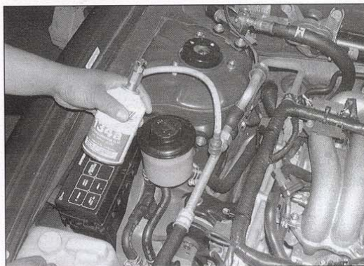
12.21 Attach the refrigerant kit to the low-side charging port - it's near the right shock tower - the cap should be marked with an "L"
