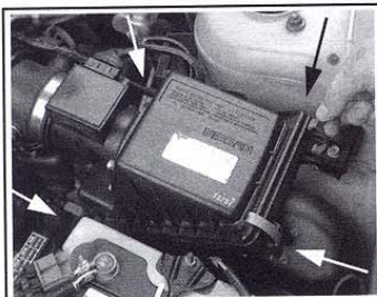
Fig. 44 The four spring clips on the edges of the air cleaner are disengaged by pulling back on the tabs
