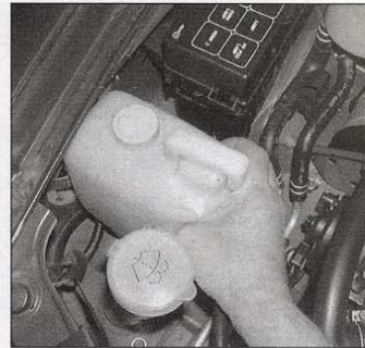
5.2 Lift the coolant reservoir straight up out of its bracket
