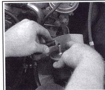
Fig. 48 Be sure the filter is in the proper direction when attaching the hoses
