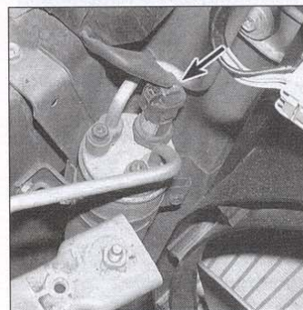
12.22 The air conditioning pressure switch (arrow) is located on top of the receiver/drier - if the compressor will not stay engaged, disconnect the connector and bridge it with a jumper wire during the charging procedure
