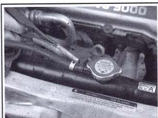
Fig. 59 Pinch the clamp with pliers to loosen it; then pull it back to remove the hose
